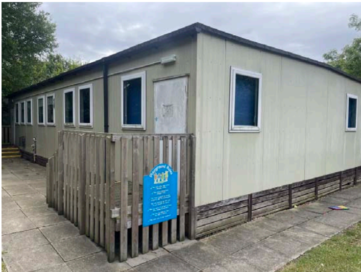
5x RLG Mobile Buildings (Elliot) 30x10ft modular cabins, 1x RLG Mobile Buildings (Elliot) 30x7ft 7" modular cabin, 3x RLG Mobile Buildings (Elliot) 28x10ft modular cabins & 2x RLG Mobile Buildings 19x10ft modular cabins configured:- 4x classrooms, library room, corridor / cloakroom, men / women / disabled toilets
