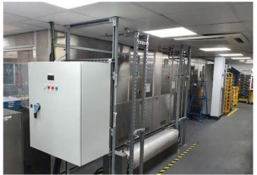
Novatec plastic wash automated line inc: 5 tanks – 1x wash detergent, 2x rinse & 2x drying, 40kHz Ultrasonic transducers on the detergent tank only in stainless steel framework, bunded trays, level switches, two-axis robot, programmed cycle times, purified water, in-line heating system. (2007) (machine ID: 0001518)
