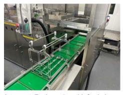
Final Clean Line 1 – Optimal Technologies Ltd robotic cleaning line, 13 tanks – 1x detergent, 7x rinse, 1x acid, 2x drying controlled by HMI & 2x currently unused, extraction is available for the acid tanks (Tank 5-8) which then passes through an acid scrubber, heaters on all tanks, 40kHz Ultrasonic transducers (2006) (machine ID: 10000500)
